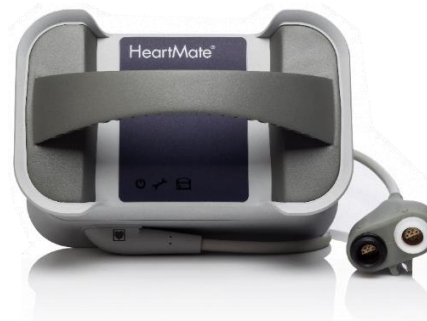
MPU (mobile power unit)
